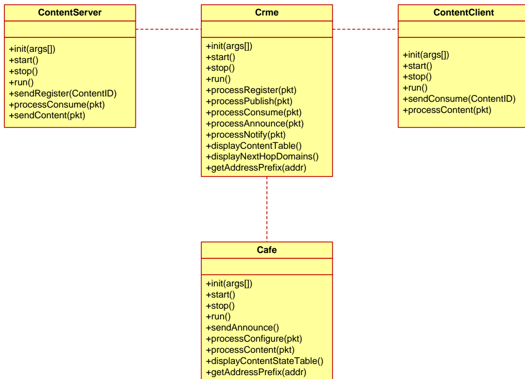
Figure 28: UML class diagram of COMET proof-of-concept emulator implementation
